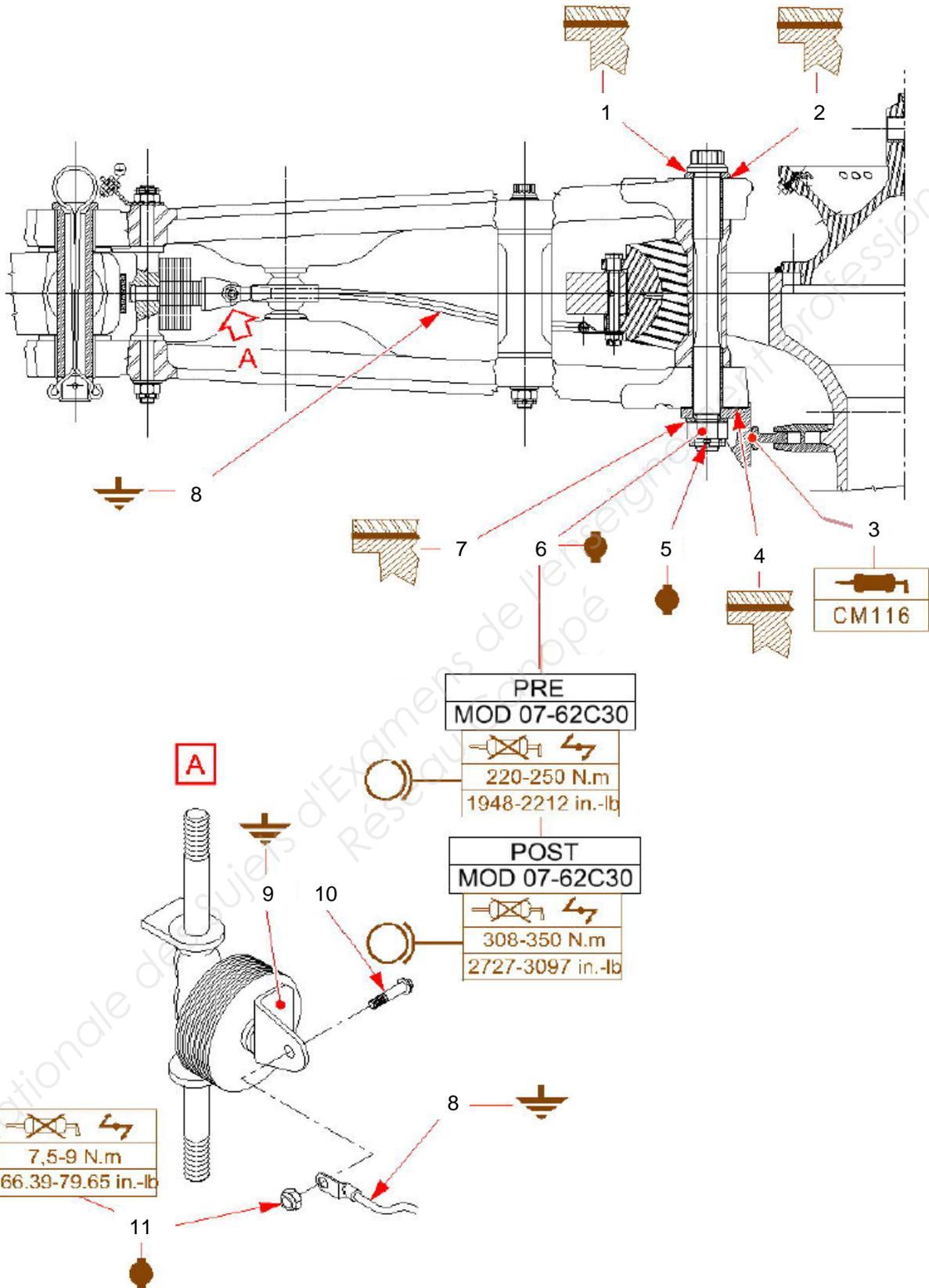
Figure 3 : Removal / Installation - Blade Sleeve Assembly (POST MOD OP62 C80)
