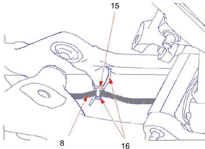
Figure 2 : Removal / Installation - Blade Sleeve Assembly (POST MOD 0762 B93)
