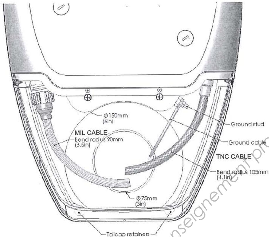
Figure 4 Cables Connected
